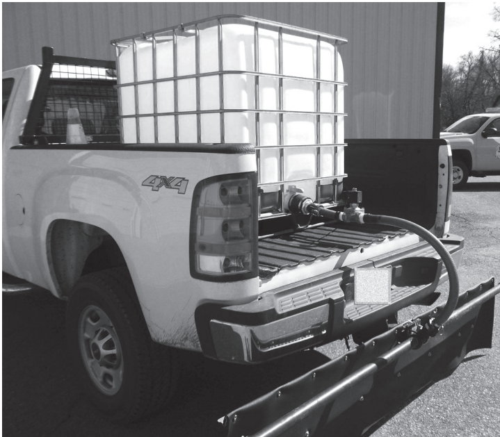
Nazareth Borough in Northampton County won the 2013 competition with its design of a storage unit to make and store brine that the public works department can apply to the borough's streets.
